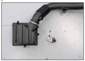
9. On vehicles equipped with a humidity sensor, remove the two screws securing the sensor into the factory air filter housing and then remove the sensor as shown.
