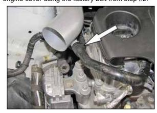
20. Connect the crank case vent hose to the fitting installed into the  $K\&N^{\mbox{\scriptsize 0}}$  intake tube.
