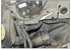
21. Remove the inner fender bolt shown.
