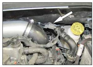
18. Connect the inlet air temperature extension harness to the factory harness.
