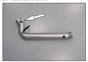
13. Install the 90° vent fitting into the grommet installed into the K&N® intake tube as shown.
