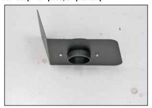
24. Install the filter adapter into the heat shield as shown using the provided hardware.
