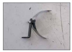
22. Assemble the saddle onto the provided bracket (070109) as shown using the provided hardware. NOTE: This step will not be used on 2017 and later Jeep Compass, skip to step #24.
