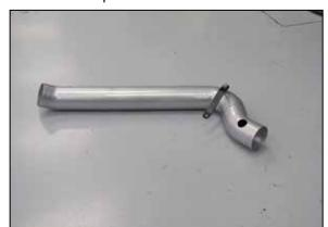
11. Install the tube mounting bracket (064335) onto the  $K\&N^{\circledcirc}$  intake tube as shown using the provided hardware.
