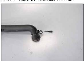
14. Remove the inlet air temperature sensor from the factory air filter housing.
